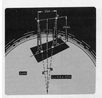
Fig. 46. Ball bearings released side by side near the earth move *closer together* as they descend. (Figure is not drawn to scale.)
