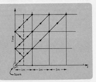
Fig. 45. Measurement of time using no clocks. Dashed line is world line of half-silvered mirror.
