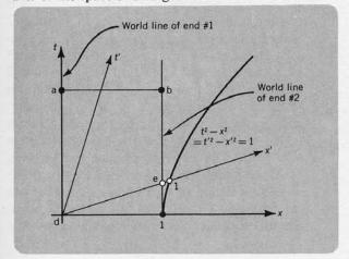
Fig. 68. A meter stick at rest in laboratory frame appears Lorentz-contracted when observed in rocket frame.
