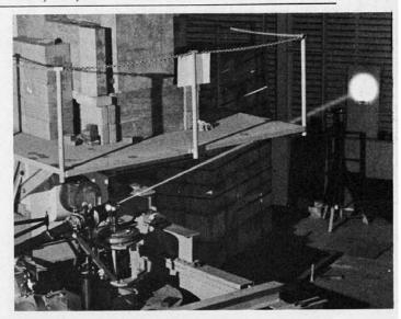
from which the calculated value of the angle is  $\phi_{\rm eale} \approx 2.4 \times 10^{-2}$  radian. The distance from exit window to screen is approximately 40 feet and the radius of the spot is about 10.5 inches, or 0.88 foot. The observed angle is thus
