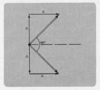
Fig. 60. Newtonian (nonrelativistic) analysis of resultant velocities in the laboratory frame after the collision.
