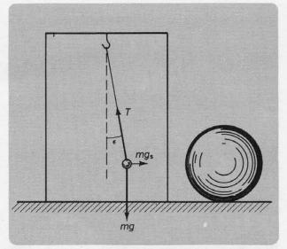
Fig. 51. Rolling the sphere to the other side results in static deflection of plumb line in opposite direction.
