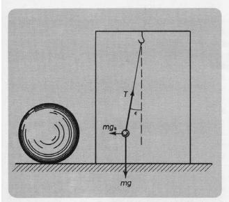
Fig. 50. Nearby massive sphere results in static deflection of plumb line from vertical.
