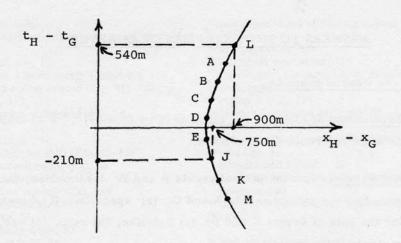
Space and time coordinates separating two events as affected by choice of frame of reference: L, laboratory frame; A, frame moving "slowly" to right relative to laboratory frame; B, C, D, ..., frames moving at higher and higher speeds to right relative to laboratory frame; J, a frame in which the coordinates happen again to be round numbers.
