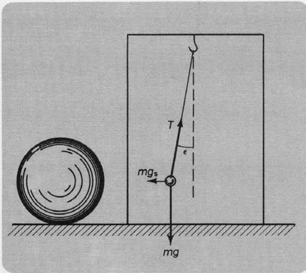
Fig. 50. Nearby massive sphere results in static deflection of plumb line from vertical.
