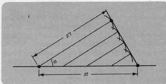
**Fig. 62.** Calculation of Cerenkov angle  $\phi$ .
