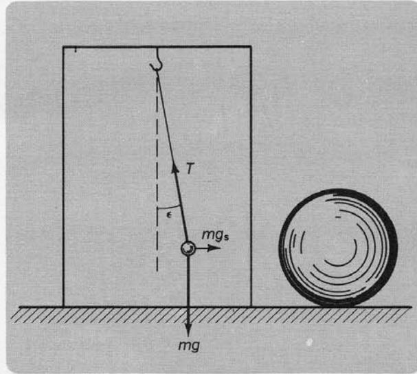
Fig. 51. Rolling the sphere to the other side results in static deflection of plumb line in opposite direction.
