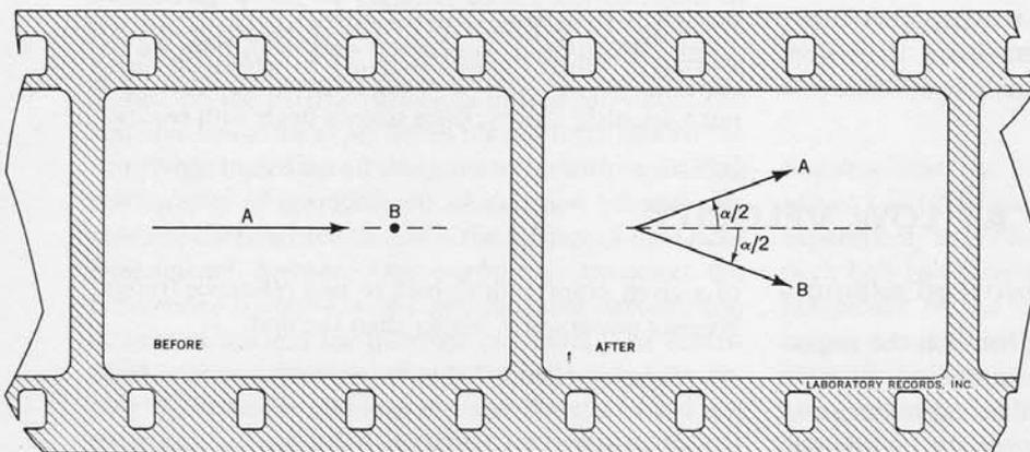
Fig. 53. Laboratory frame record of a symmetric elastic collision.
